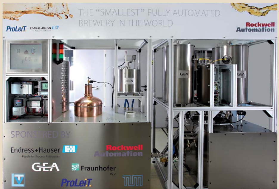
Fig. 1 Mini-brewery with two-kettle brewhouse and fermenting cellar
