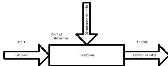
**Figure 1: Controlled system**
