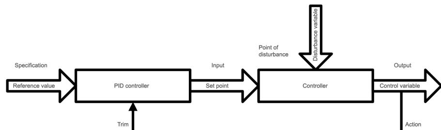
**Figure 2: Controlled loop**
