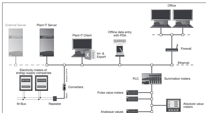
Fig. 1: All the energy meters – the energy and consumption-relevant real-time data from the process control system (bottom right), the meters of the respective utility companies (bottom left) and the offline meters through use of PDAs – are integrated in a common data pool
