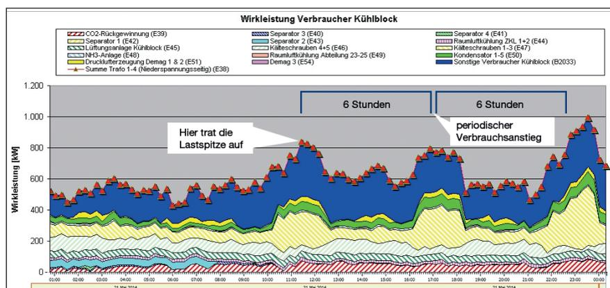
Fig. 4 and 5: Starting up a cooling system at the same time as other processes can result in expensive load peaks; strategies in the energy management can prevent the simultaneous operation of energy-intensive units – without any negative impact on the process.
