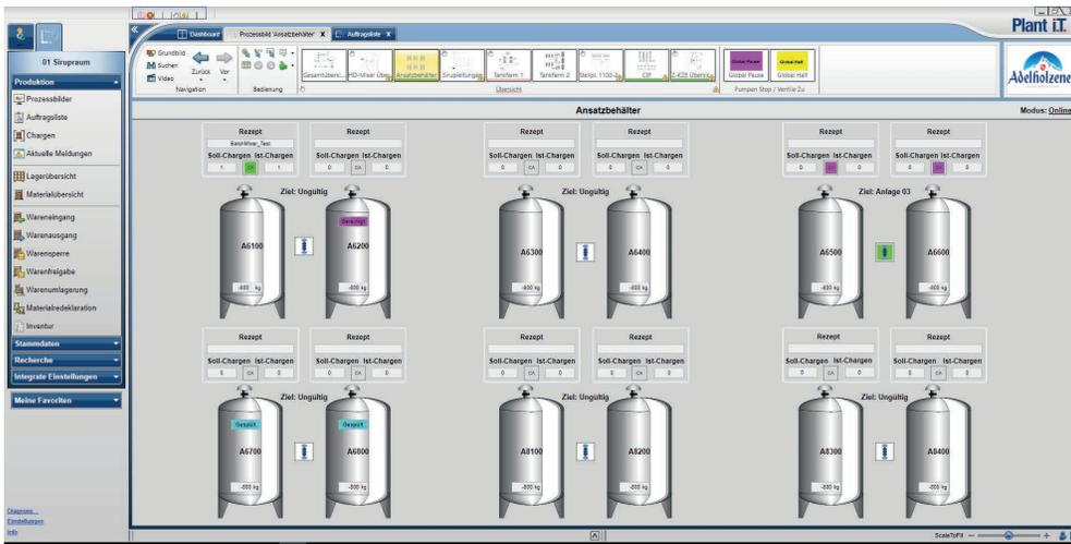
Plant Batch iT – process image of the preparation tanks
