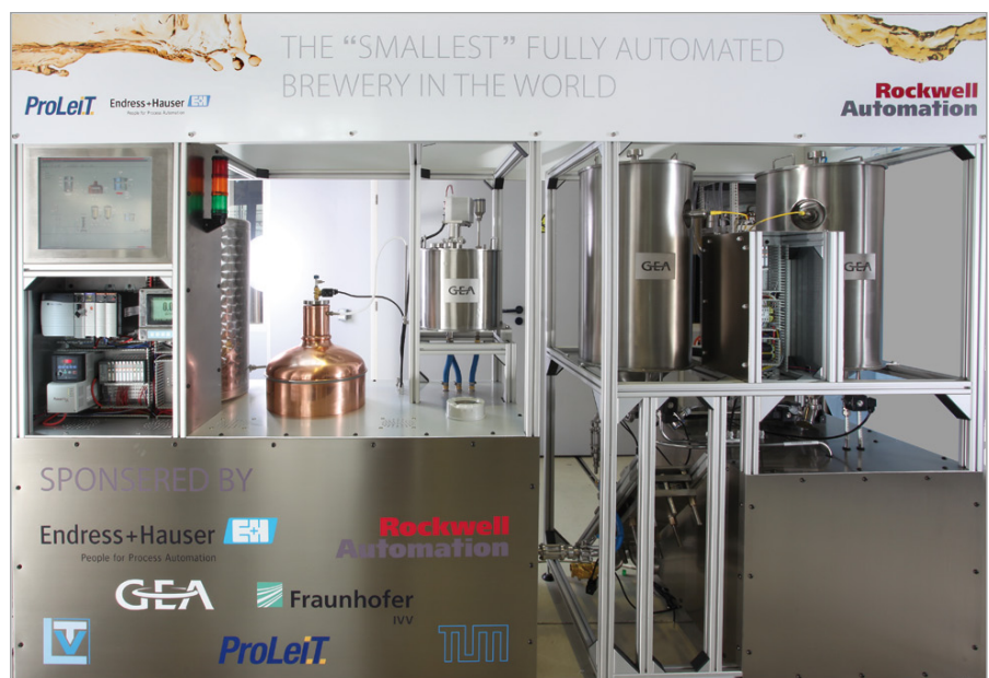
The smallest fully automated brewery with a two-vessel brewhouse system and a fermentation cellar
