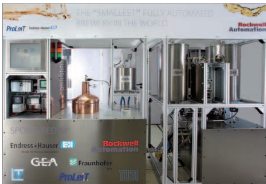
The smallest fully automated brewery with a two-vessel brewhouse system and a fermentation cellar
